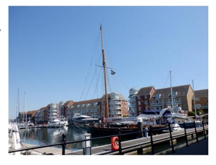
In numbers, *Carlotta* is in the mid-range of BPCs. Built in 1899 she is fifty feet (15m) in length, not including bowsprit; has a beam of thirteen feet and draws eight feet. She weighs 28 tonnes.
