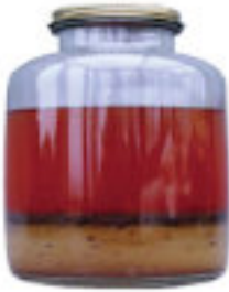
Fig.1 Shows diesel bug growth trapped in pre-filter cyclones
